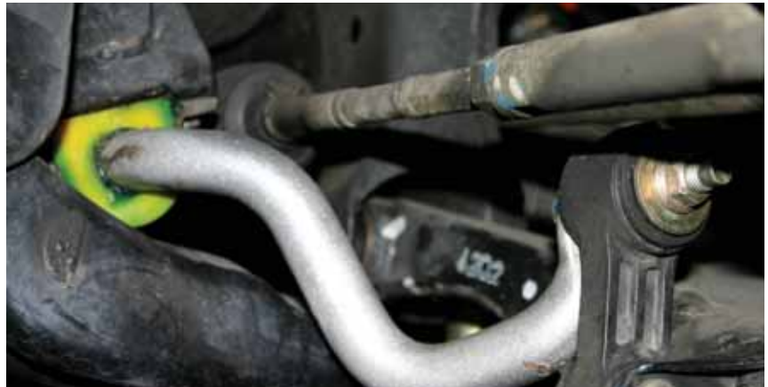
TWO-POSITION ADJUSTABLE AND INCLUDES NEW URETHANE SWAYBAR BUSHINGS. WE SUBSTITUTED LONGER LASTING BLUE MARINE GREASE INSTEAD OF THE INCLUDED WHITE LITHIUM GREASE.
