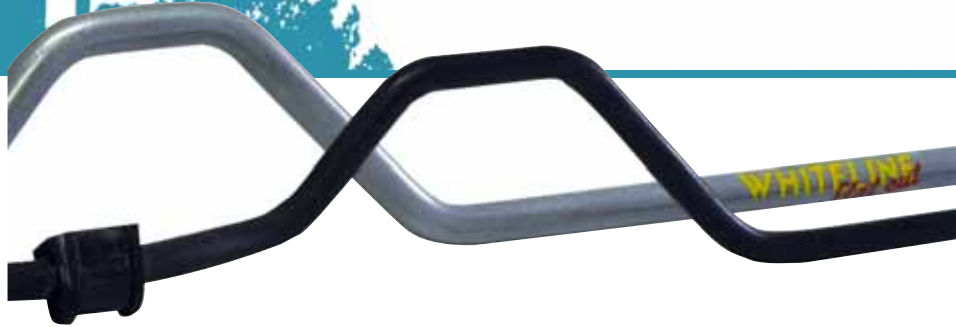
THE DIFFERENCE IN THICKNESS BETWEEN THE STOCK BAR AND THE WHITELINE BAR IS IMMEDIATELY OBVIOUS
