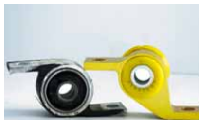
THE OFFSET BETWEEN THE WHITELINE ALK AND THE STOCK CONTROL ARM BUSHING IS OBVIOUS. OUR ALK CAME EQUIPPED WITH A URETHANE BUSHING VS. THE STOCK RUBBER MATERIAL.
