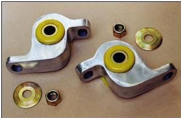
An anti-lift kit and an adjustable rear bar - definitely.
