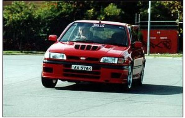
Nissan's Pulsar GTi-R needs shocks badly. Their weight distribution is horrendous - it's the worst. You really benefit from better front shocks to control the front end from oscillating, maintaining contact between the tyres on the road.
