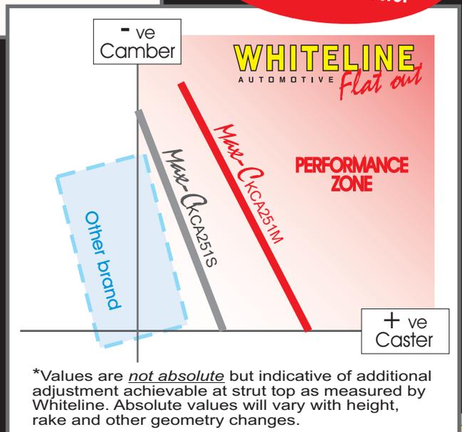
\*Values are *not absolute* but indicative of additional adjustment achievable at strut top as measured by Whiteline. Absolute values will vary with height, rake and other geometry changes.
