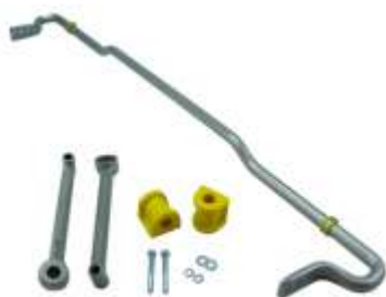
BSR49XXZ REAR SWAY BAR 24MM 3 POINT ADJUSTABLE WITH SUPPORT BRACE
