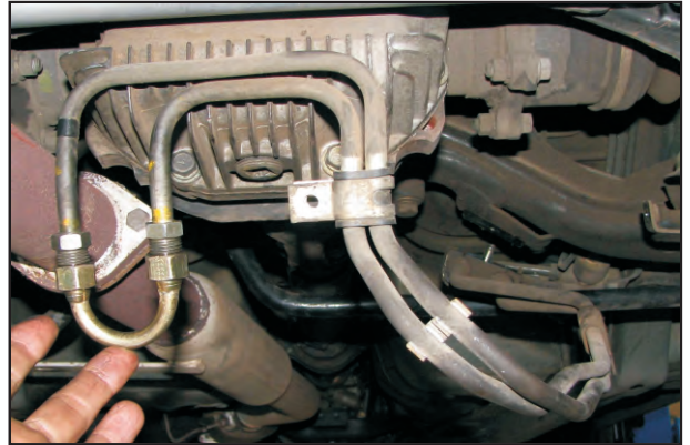
Photo 1: Hydraulic By-pass pipe
