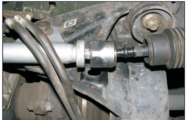
Photo 2: Inner tie-rod fitment
