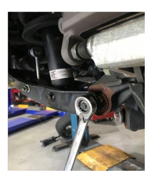
Proceed to remove rear lower control arms -Disconnect swaybar link and lower shock bolt.
