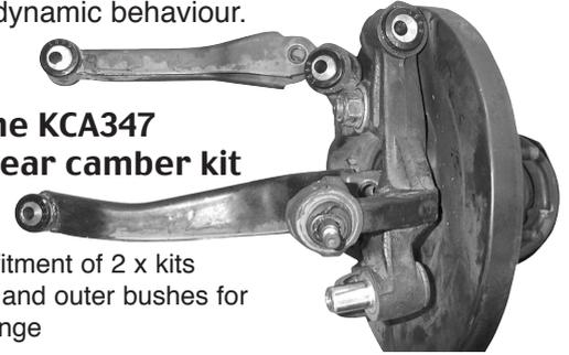
Picture shows fitment of 2 x kits replacing inner and outer bushes for 1.5 degree change
