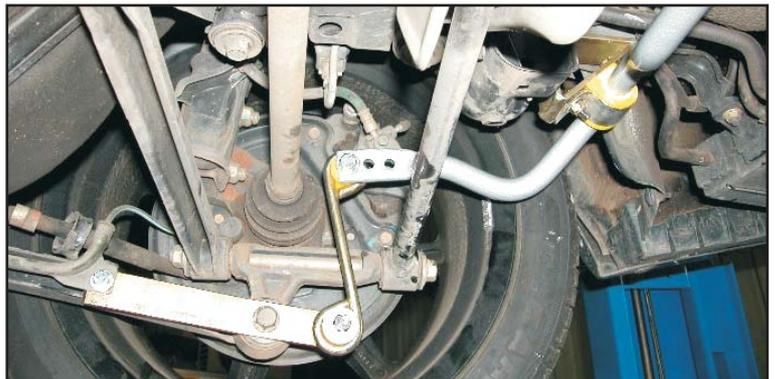
Photo 5. BSR47Z complete assembly - right hand side shown.
