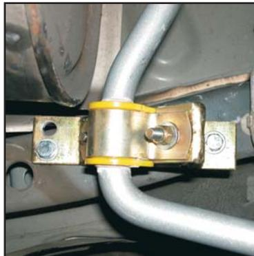
Photo 1. BSR47Z - chassis mount left hand side - bottom view.
