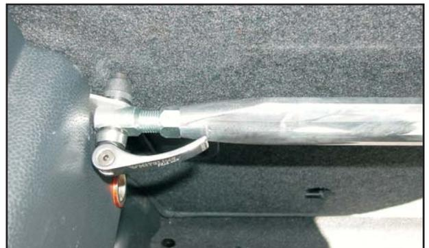
Fig 3. Quick release mechanism.
