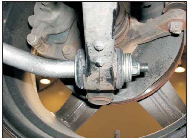
Fig.1. BSF90 - right-hand side, max positive caster adj.
