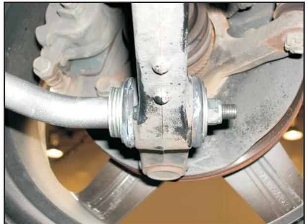
Fig.2. BSF90 - right-hand side, max negative caster adj.
