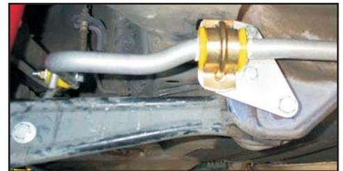
Fig. 4 Chassis bracket assembly
