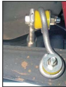
Fig. 2 Swaybar link assembly
