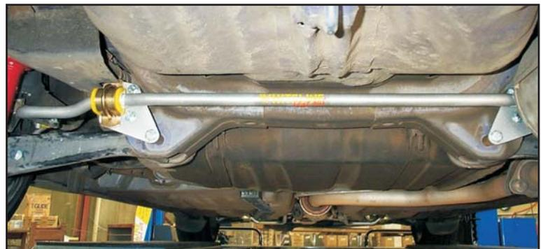
Fig. 6 Complete swaybar assembly
