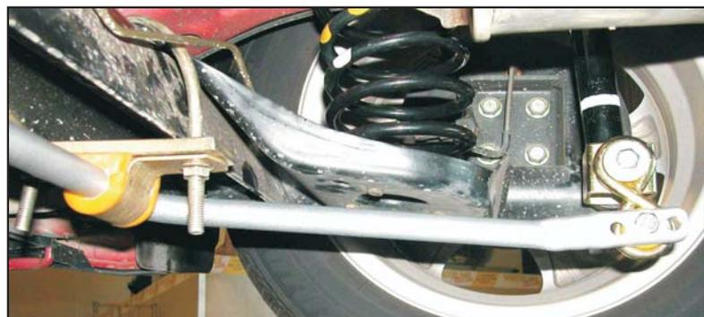
Fig. 4: Swaybar assembly
