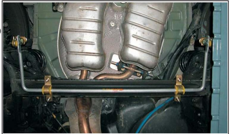
Fig. 2: Complete Swaybar assembly
