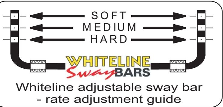
Fig. 1: sway bar adjustment guide.
