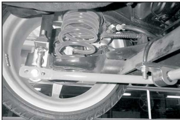
Fig.3. BHR73Z axle and link mount, set to middle adj.
