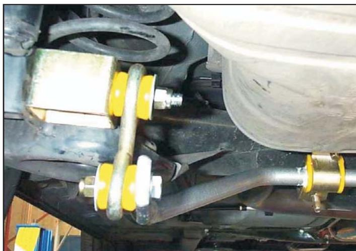
Fig. 3 Left hand side swaybar link assembly
