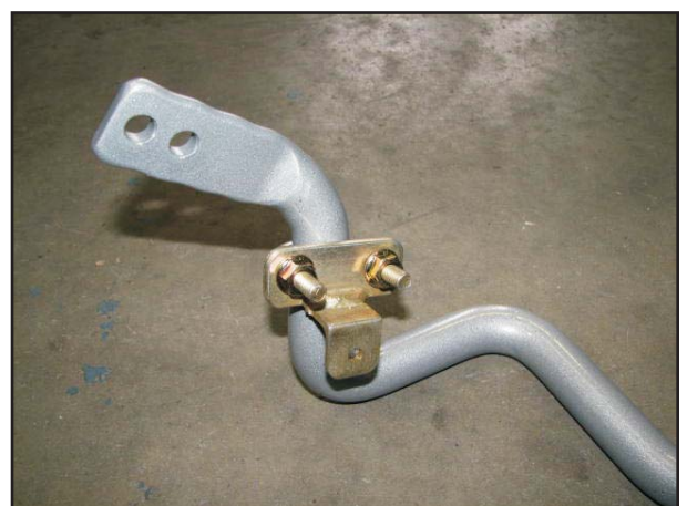
Photo 2. Whiteline Swaybar ride height sensor mounting bracket
