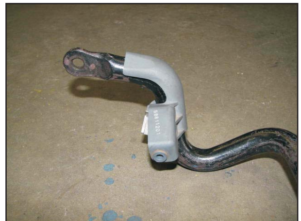
Photo 1. OEM Swaybar ride height sensor mounting bracket
