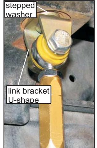
Photo 2 - Upper Link bracket as fitted to GU front.
