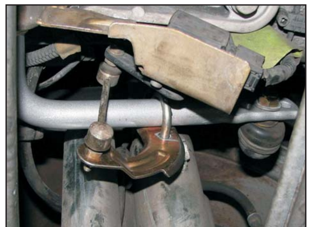
Photo 2. Whiteline swaybar with ride height sensor locating bracket
