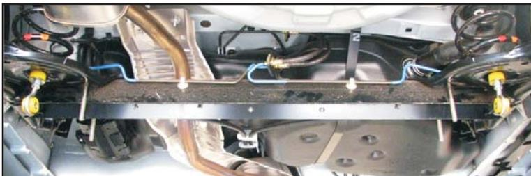
Photo 3. Link assembly and U-bolt - bottom view.
