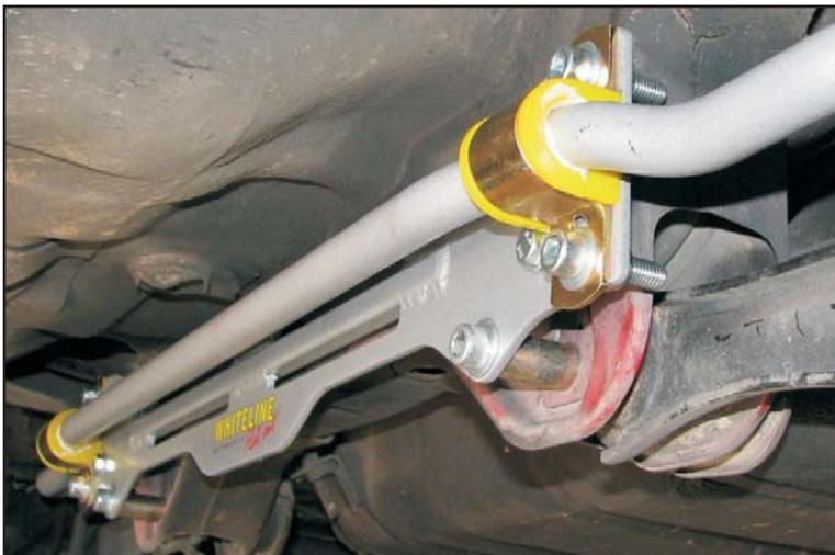
Photo 3. KBR17-22 complete assembly - side view.
