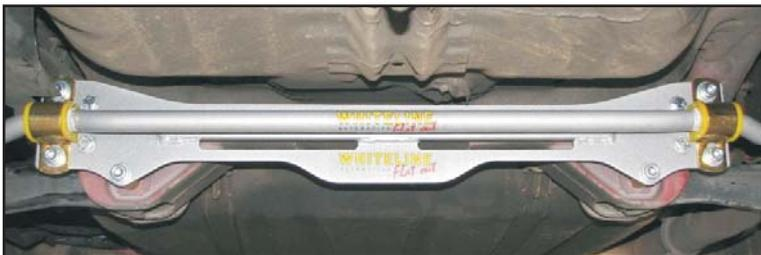
Photo 4. KBR17-22 complete assembly - rear view.
