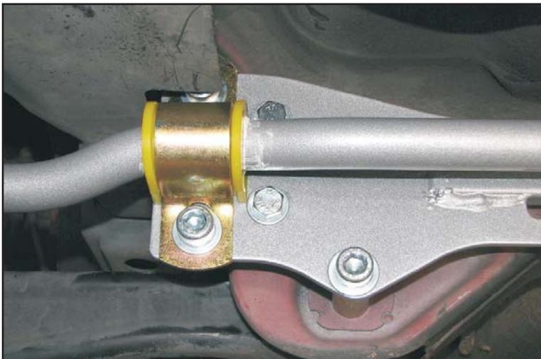
Photo 2. Swaybar mounting - left side.
