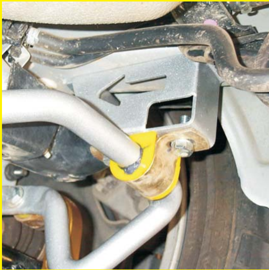
Right hand side looking out from centre towards front. Arrow points toward front of vehicle to simplify fitting. Note new cut-out for extra clearance for larger mufflers. (when used on left hand side)
