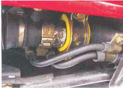
Whiteline's steering rack bushings make such a shocking improvement in steering feel..
